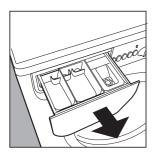
The detergent dispenser can be removed and cleaned: pull it outwards, as indicated in the figure. Then leave it under running water for a few minutes.
